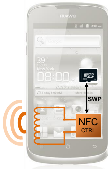
Figure 4: SWP microSD memory card solution
