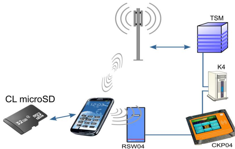
Figure 5: Contactless access control system infrastructure overview
